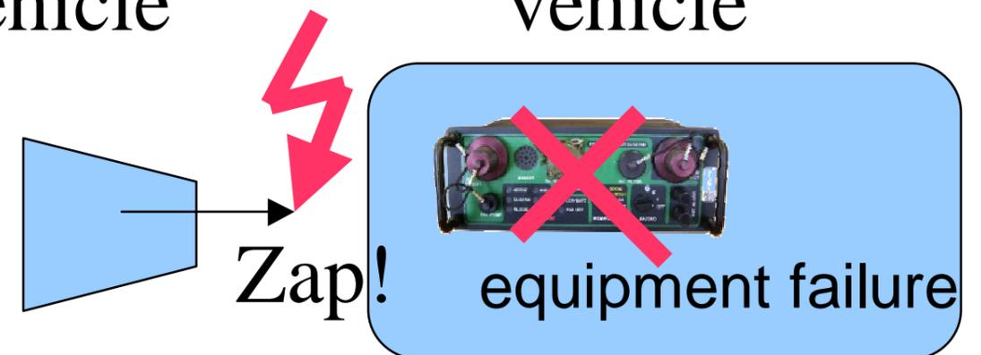
Due to spacecraft charging, severe Electrical discharges can happen during different space operations leading to critical equipment failures in orbit
